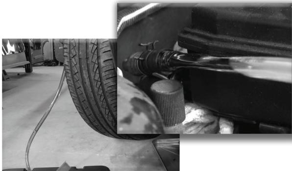
**6.** Top off the reservoir with new power steering fluid. Then with the car running, turn the steering wheel from full left to full right a couple of times. This will begin to flush the fluid.
